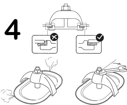
Do not over-tighten as it will over-compress the gasket and shorten its service life. If the gasket leaks while pressure is being built up, tighten only enough to stop leakage. This prevents the vaccum that's developed by cooking on a shut down from pulling in and draining the boiler.
